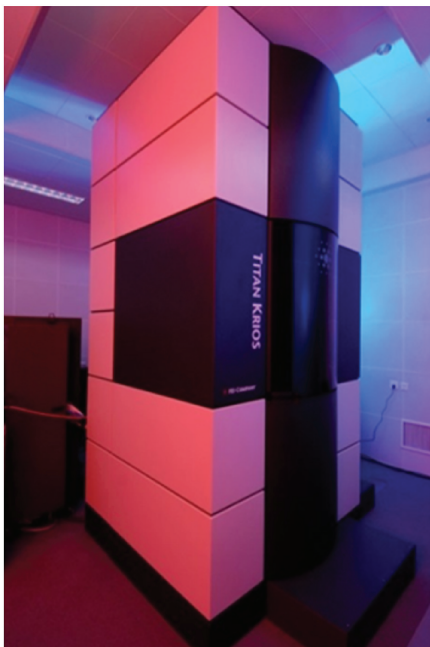
Fig. 3 Thermo-Fisher Titan Krios electron microscope (left); Electronic-optical system of Titan Krios (right)
